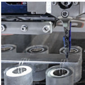
Wire bonds on 18650 battery cells
