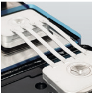
Prismatic cells connected by aluminum ribbons
