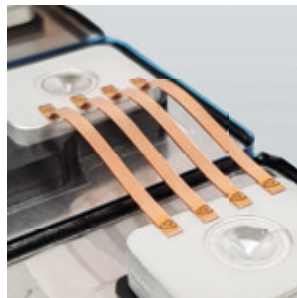
Prismatic cells connected by copper ribbons
